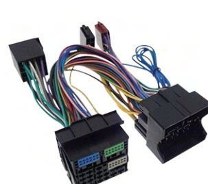
GZCS ISO QUADLOCK I Quadlock to ISO connector GZCS ISO QUADLOCK II Quadlock II to ISO connector
